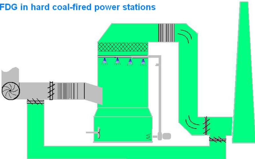
**Green section:** Possible areas for use of cost-optimized plates roll-cladded with alloy 59 with a minimum cladding thickness of 1.5 mm. **Grey area:** Further areas of application to be agreed upon in accordance to the particular plant situation.
